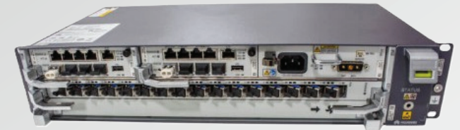
OLT X2 (XGPON/GPON)
